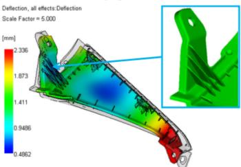
We suggested that thickness and the total length of the ribs must be increased in order to minimize warpage and get better results.
